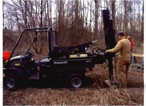
Figure 2: Geo-probe equipment in action for a Phase II, CRM-based study along a first terrace location of the Delaware River, eastern Pennsylvania.
